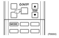
Note: When the remote controller is left untouched for 60 seconds, it returns to the normal mode.
