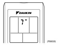
9. Press the **ON/OFF** button twice to return to the normal mode.
