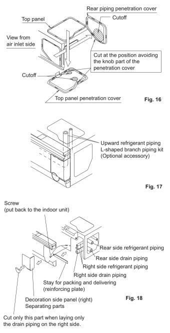
After piping is finished, cut the removed penetration cover along the shape of piping, and install it.
