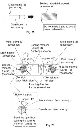
· Be sure to insulate all drain piping running indoors.
