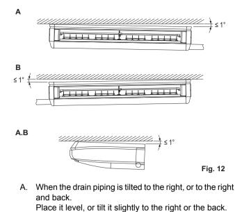
(Within 1°) B. When the drain piping is tilted to the left, or to the left
