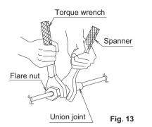
• When making a flare connection, coat the flared inner surface only with ether oil or ester oil. (Refer to Fig. 14) Then, turn the flare nut 3 to 4 times with your hand and screw in the nut.
