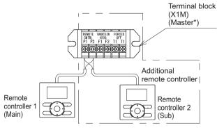
\* For simultaneous operation system, be sure to connect the remote controller to the master unit. Fig. 37
