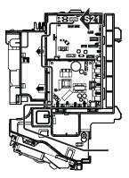
**3** Put the electrical wiring box cover back and pull the wire harness around it as shown in the figure above.
