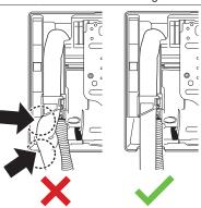
2 Pass the drain hose and refrigerant piping through the wall hole and seal the gap with a putty.
