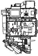
Put the electrical wiring box cover back and pull the wire 3 harness around it as shown in the figure above.
