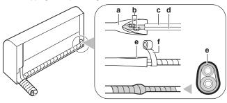
a Heat insulation pipe cover (on the indoor unit side)b Flare connections
