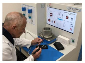
All modifications are tested in the explosive atmosphere of the spark-test apparatus for intrinsically safe circuits
