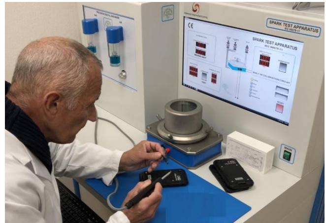
All devices are tested in the explosive atmosphere of the spark-test apparatus for intrinsically safe circuits
