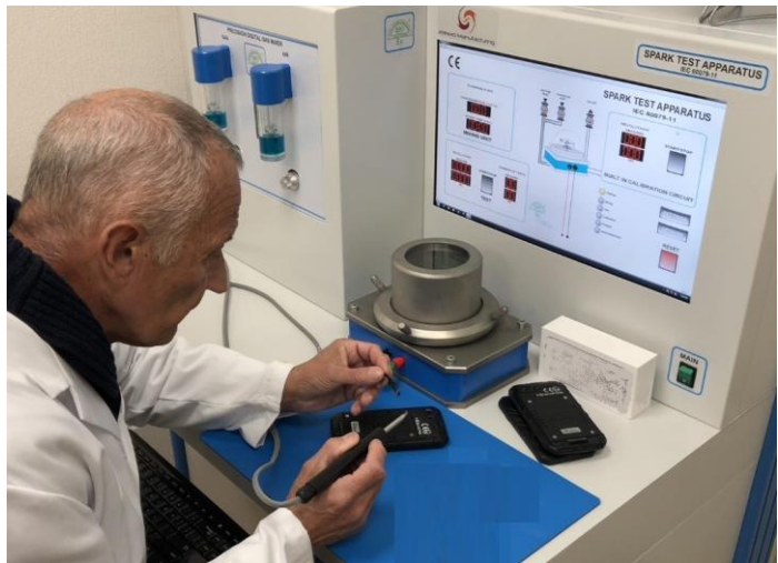
All devices are tested in the explosive atmosphere of the spark-test apparatus for intrinsically safe circuits
