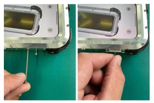
2. Use the Apple tool to unlock the simcard holder and use the paperclip (C) to remove it
