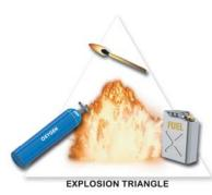
So that an explosion can occur, three conditions must be fulfilled; see the explosion triangle diagram.
